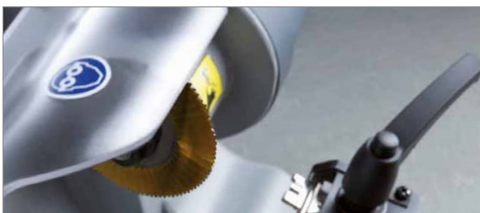
TiN-coated cutter with side cuts
