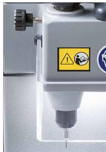
Spring loaded tracer point
