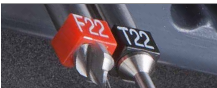
Cutting tools with identification collar
