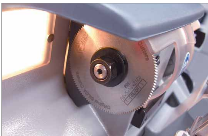
Prismatic cutter made of HSS
