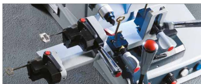
Omnia W-Max: vertical cuts carriage
