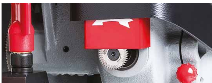
Cutter for internal cuts
