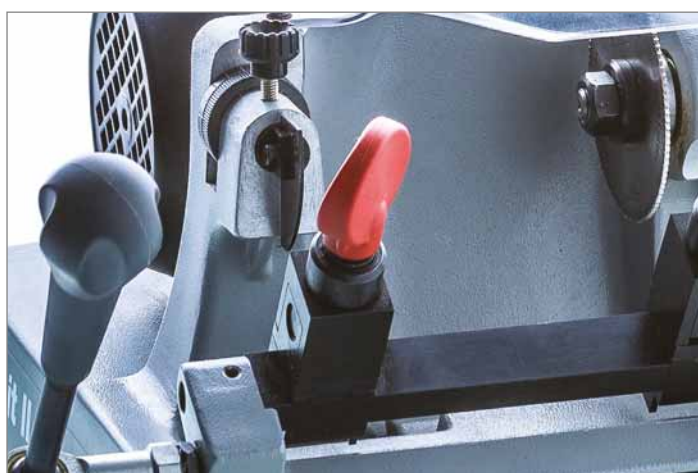
Spring loaded tracer point
